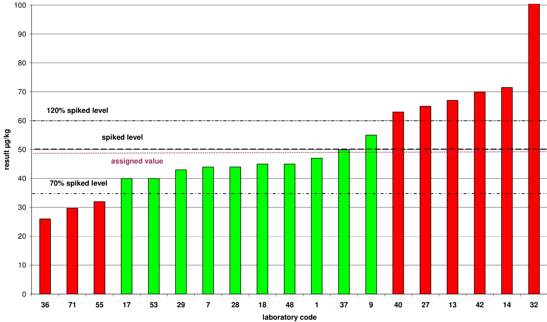
Figure 5: Assessment of Fenitrothion (spiked level: 50 µg/kg) in Parsley Purée Test Material A
